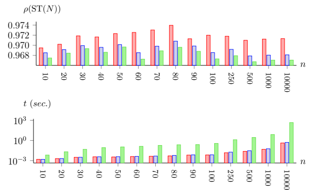
Figure 5: Averaged ratios and CPU times for ESTEIN instances in \mathcal{R}^2 . DM (red), DB (blue), GeoSteiner (green).
