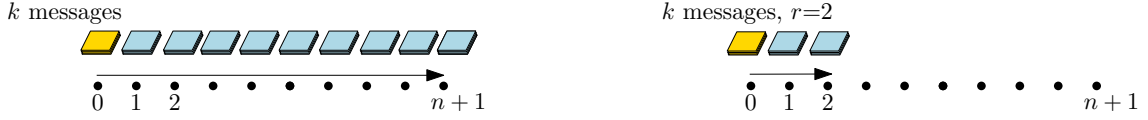
Figure 1: Illustration of the scenarios. Left: with unbounded reach, the k messages arrive immediately to all nodes, but that does not prevent intermediate nodes from forwarding the messages. Right: with range r = 2 , the messages sent from node 0 only reach up to node 2, so forwards are necessary to reach the target, n + 1 .
